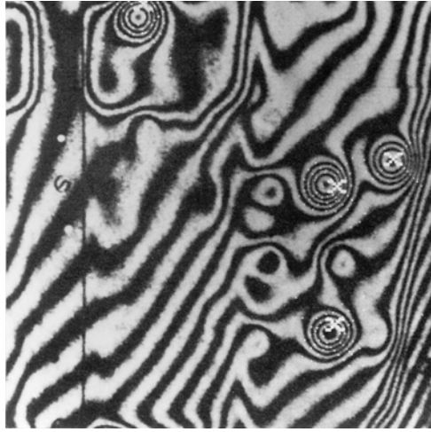
Figure 13.1. Holographic interferogram of a honeycomb panel, showing sites of poor bonding (D. W. Robinson, Appl. Opt. 22 , 2169–2176, 1983).
